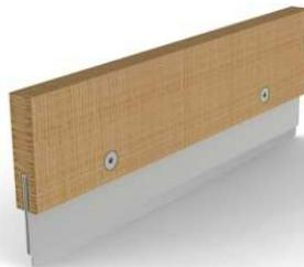
Spread solder paste on the back end of the stencil. Move the squeegee towards you to push the paste into all stencil openings. Push the squeegee down firmly and move forward in one fluent movement.
