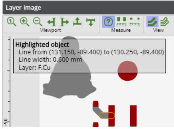
The information contains the shape and position info along with the layer on which the object is found.
