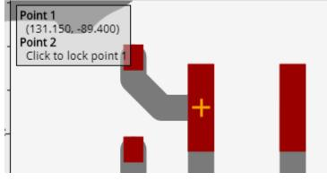
Then move the mouse to define a second point. The coordinates of both points are displayed together with the distance between both points. Using this method it is possible to measure e.g. the pitch of a component.
