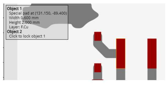
Then move the mouse over the second object. Information about both objects is displayed together with the clearance between both objects.
