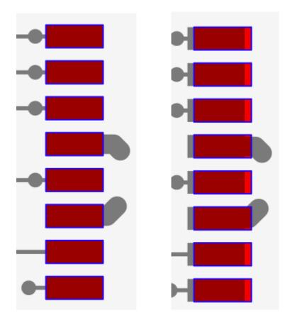
If you also selected the corresponding copper layer as extra layer, if the Solderpaste data that overlaps with the copper data will be shown in dark red otherwise, it is shown in bright red.
