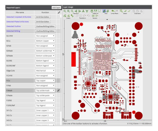
For smaller or lower resolution screens, you are able to fold away the Material and Buildup view panels to make more space for the Layer Image.
